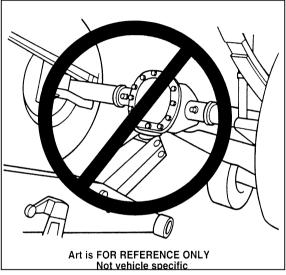
The improper lift point
